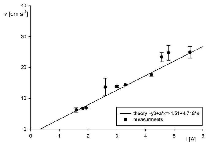
Fig 2 Terminal velocity vs battery's current
